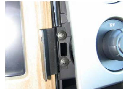
Bottom part of InDash installed. Notice clip location.
